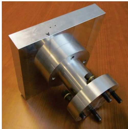
Fig. 2 Cylindrical concept fixture with a 7 x 1.25 inch square plate to simulate loading with a small test article.
