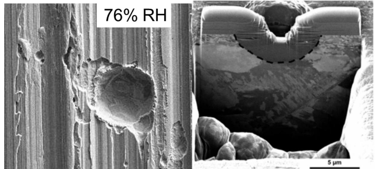
Weirich, T. D., Srinivasan, J., Taylor, J. M., Melia, M. A., Noell, P. J., Bryan, C. R., ... & Schindelholz, E. J. (2019). Humidity effects on pitting of ground stainless steel exposed to sea salt particles. *Journal of The Electrochemical Society*, 166(11), C3477.
