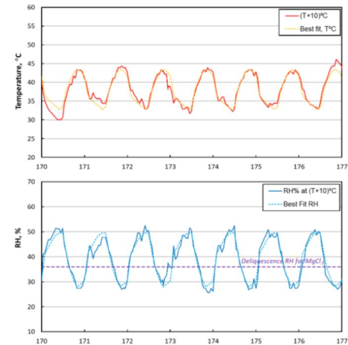
*Cyclic atmospheric conditions developed from Arkansas Nuclear 1 ISFSI (SNL 2021 M2)*
