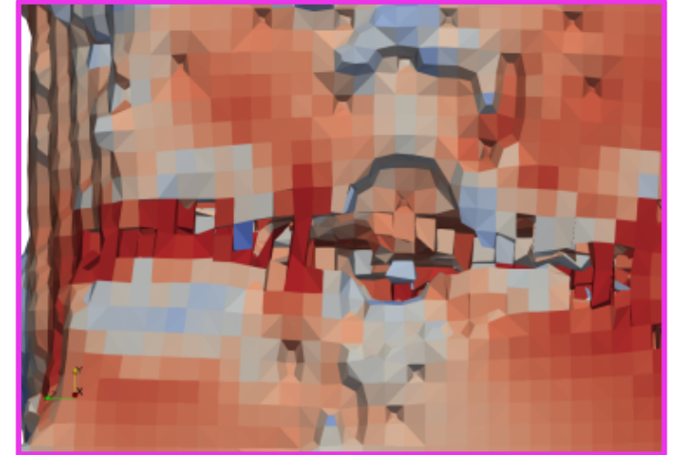
Strain and failure localization along the edge was correctly predicted from high-fidelity modeling
