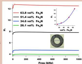
VSM measurements on 75.3 vol% Fe<sub>4</sub>N/NND revealed a saturation magnetic polarization of  $J_s = 1.19$  T, which lies between silicon steel ( $J_s = 1.87$  T) and ferrite ( $J_s \sim 0.5$  T). Polarization ( $J$ ) is related to magnetization ( $M$ ) by the equation  $J = \mu_0 M$ . Magnetization measures atomic magnetic moment density. Therefore, Fe<sub>4</sub>N/NND SMCs surpass the magnetization of common permanent magnets and approach conventional soft magnetic materials.
