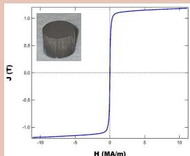
Optimal magnetic properties will be sought with higher vol% loading of Fe<sub>4</sub>N in the epoxy. Prototype motor parts will be made from the Fe<sub>4</sub>N/NND composite.
