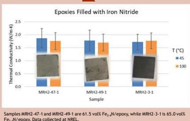
nitride in TTE SMCs showed thermal conductivities in the range of 1.5 to 2.0 W/(m·K). Further measurements are underway on neat NND and 65 vol% iron nitride/NND composites cured at high temperature (i.e. 255 °C).
