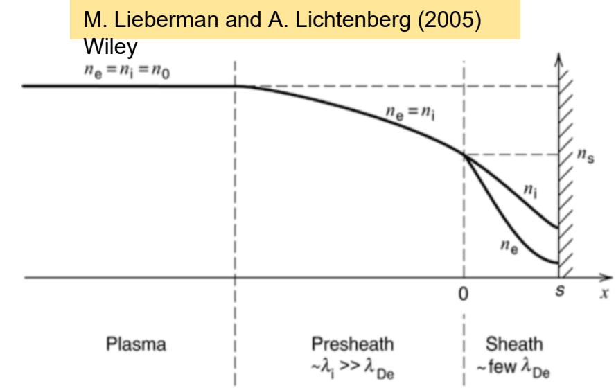
$$\Gamma_w = a_l h_l n_0 c_{s,c} \quad c_{s,c} = \sqrt{T_{e,c}/m_i} \quad a_l = \frac{V_{i,se}}{c_{s,c}} \quad h_l = \frac{n_{se}}{n_0}$$
