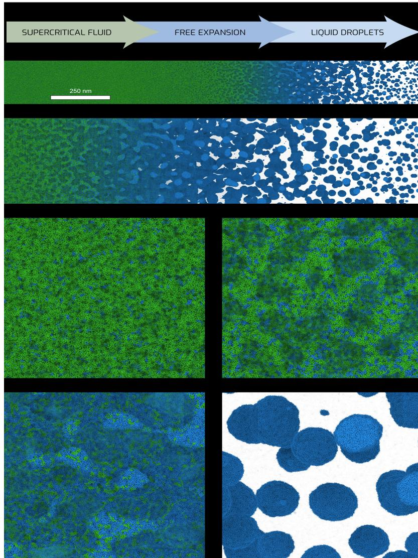
**LAMMPS molecular dynamics simulation of supercritical aluminum (green) expanding into the liquid/vapor two-phase region (blue), resulting in spinodal decomposition and coalescence of liquid droplets. The simulation used ~1.5 billion atoms running on 8,192 GPUs (47% of NNSA's ATS-2 Sierra supercomputer). Aluminum was modeled using the SNAP machine learning interatomic potential, trained with quantum chemistry calculations.**
