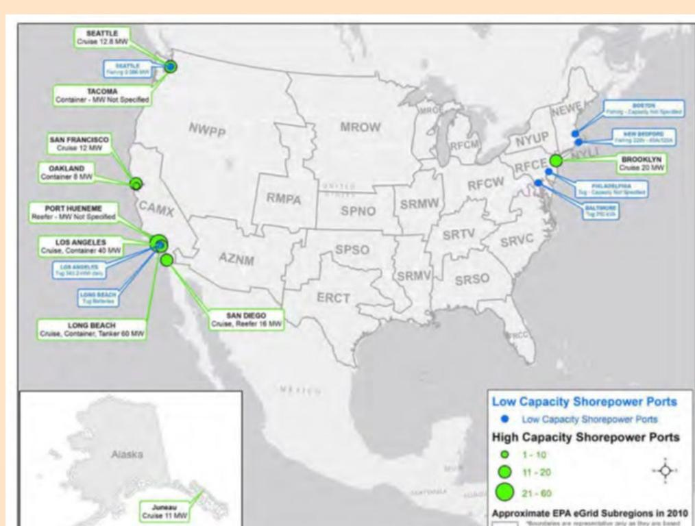
Shore power allows for a vessel to plug into the local grid while at-berth, as opposed to running its auxiliary engine
