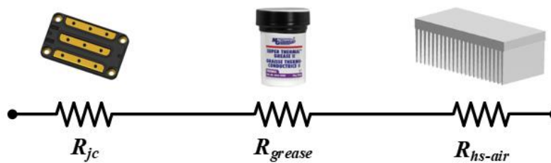
(c) SiC module thermal equivalent model
