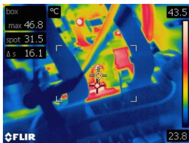
(c) PCB surface temperature rise under 200 kW
