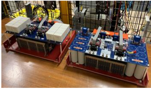
(a) primary and secondary power stage
