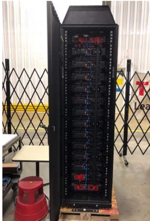
(b) Battery cabinet and wired batteries
