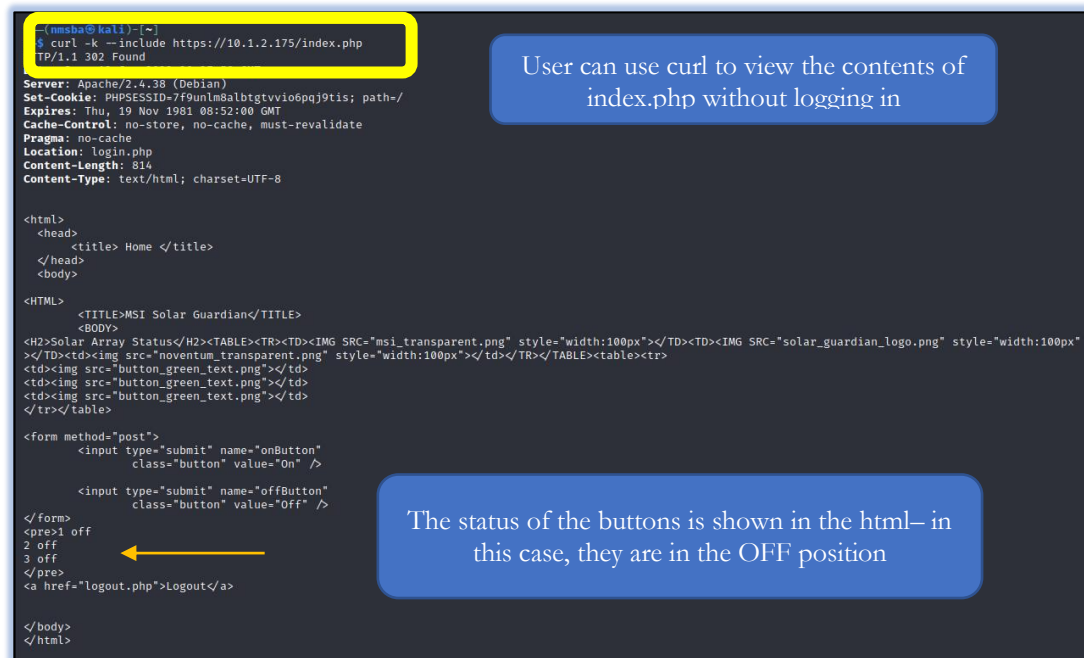
Figure 5: Using curl, an unauthenticated user can view restricted content on index.php
