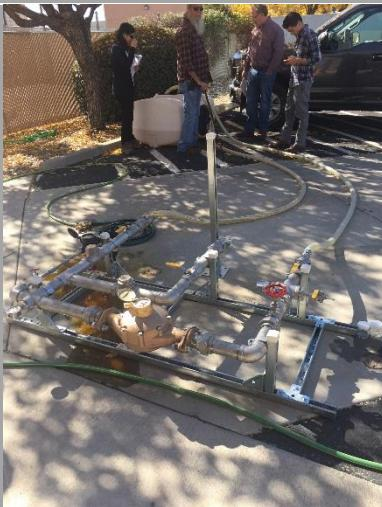
A photograph showing a complex stainless steel piping manifold on a concrete surface. A sump pump unit is visible in the background. Several people are standing around the setup, and a white drum is nearby.                             | <p><b>Field Condition Setup</b></p> <p>Premix tank with Sump Pump is shown in background. Main manifold is shown in foreground. Water is recirculated through the main manifold from and back to the premix tank.</p> |
