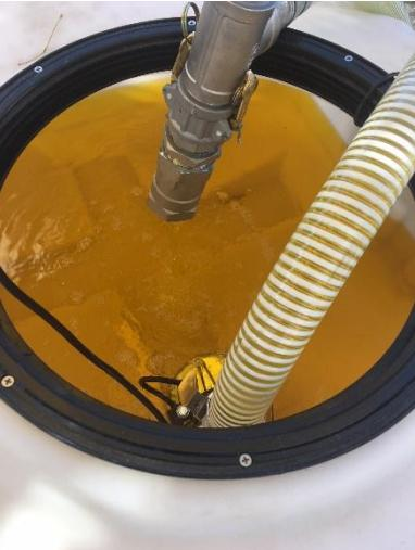
A photograph showing a close-up of a hose connected to a large black tank. The tank is filled with a yellow liquid. The hose is being used to recirculate the dye at the premix tank.                                  | <p><b>KB-1 Dispenser Simulation Recirculation of Dye at Premix Tank</b></p> <p>During the KB-1 Dispenser Simulation the test water was dyed yellow confirming that the KB-1 sidestream is functioning as designed.</p>                               |
