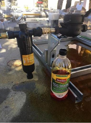
A photograph showing the KB-1 Dispenser Simulation Setup. It includes a proportioning injector connected to a yellow dye bottle labeled 'DURKES EGG SHAPER' and a flow totalizer. The setup is mounted on a metal frame. | <p><b>KB-1 Dispenser Simulation Setup</b></p> <p>The KB-1 Dispenser Simulation Setup including the proportioning injector, yellow dye, and flow totalizer are shown.</p>                                                                             |
