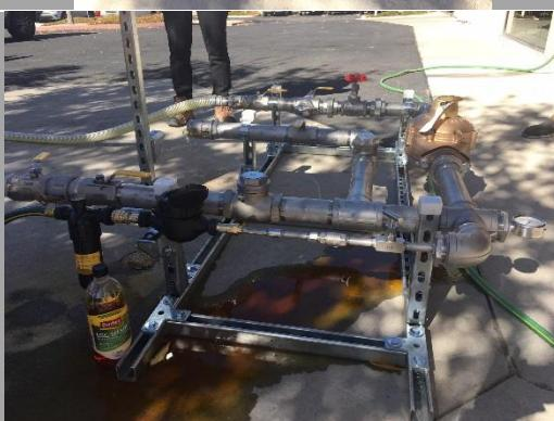
A close-up photograph of the main manifold. A large copper-colored KB-1 dispenser simulation component is connected to the manifold. A bottle of yellow tracer dye is placed next to the setup. The manifold is mounted on a metal frame. | <p><b>Main Manifold with KB-1 Dispenser Simulation Setup</b></p> <p>The KB-1 Dispenser Simulation Setup is shown connected to the KB-1 Sidestream connection on the Main Manifold.</p>                                |
