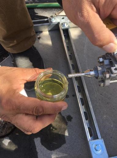
A photograph showing a hand holding a small glass jar filled with yellow liquid. The jar is being held over a metal tray, and a dispensing nozzle is being used to fill it.                                             | <p><b>KB-1 Dispenser Simulation Sample</b></p> <p>During the KB-1 Dispenser Simulation a sample was collected at the Main Manifold sample port SPT. The yellow color in the sample confirms that the KB-1 sidestream is functioning as designed.</p> |
