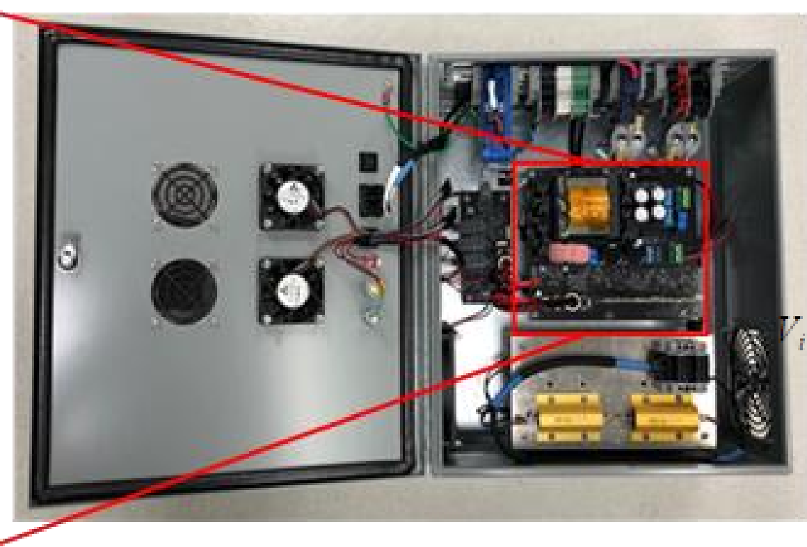
Custom-designed and built switch-mode power converter used to stress GaN and SiC WBG power devices
