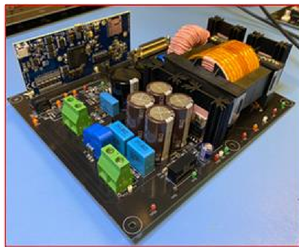
Custom-designed and built switch-mode power converter used to stress GaN and SiC WBG power devices
