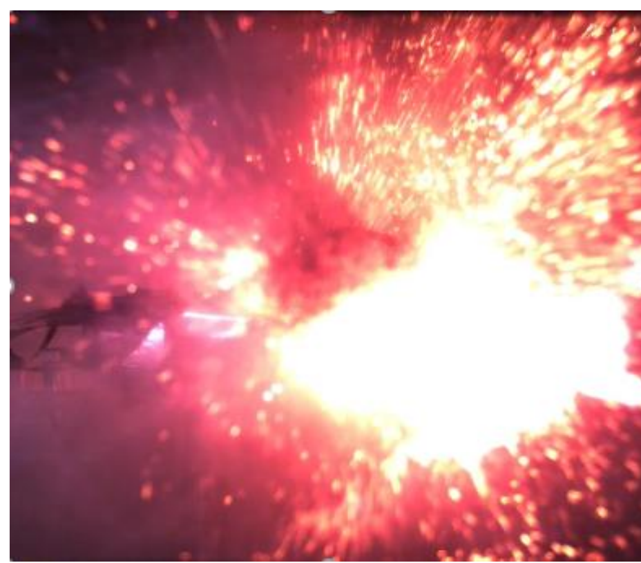
Figure 1: Failing 18650 format cell
