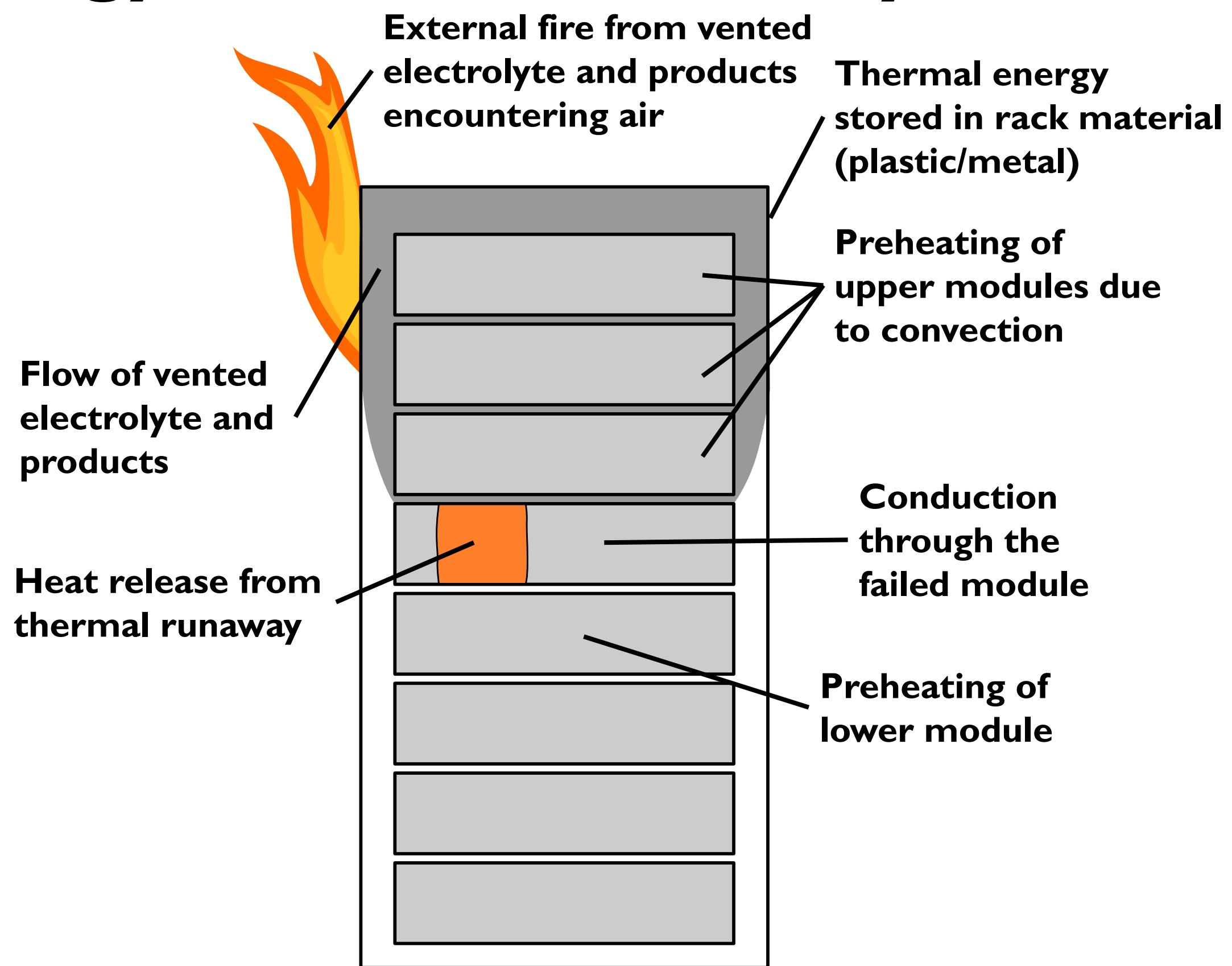
Thermal energy conservation module  $i$  in a network of  $N$  modules:
