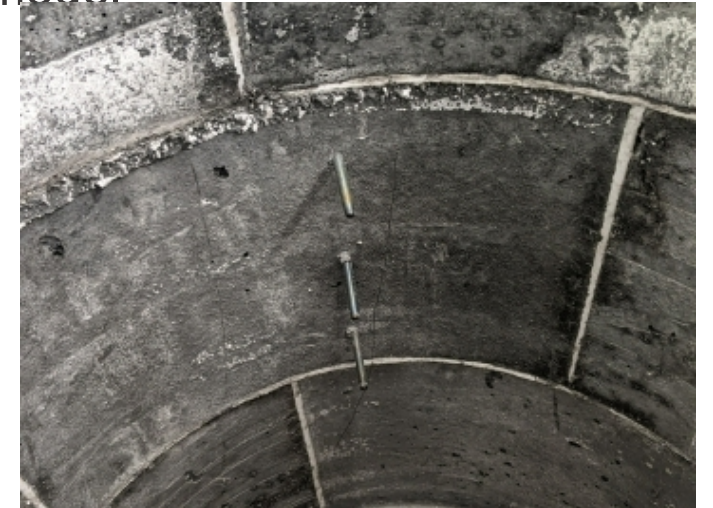
Thermocouples in test bin
