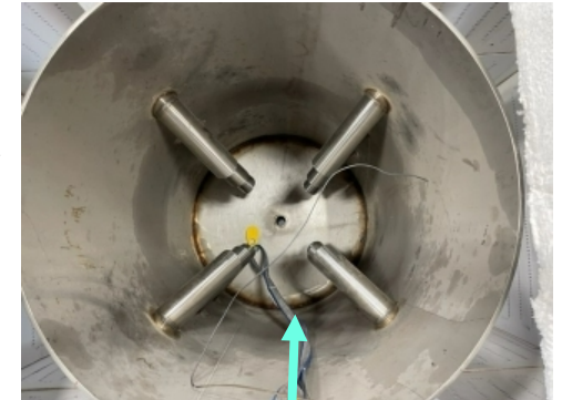
charging bin with heat transfer tubes
