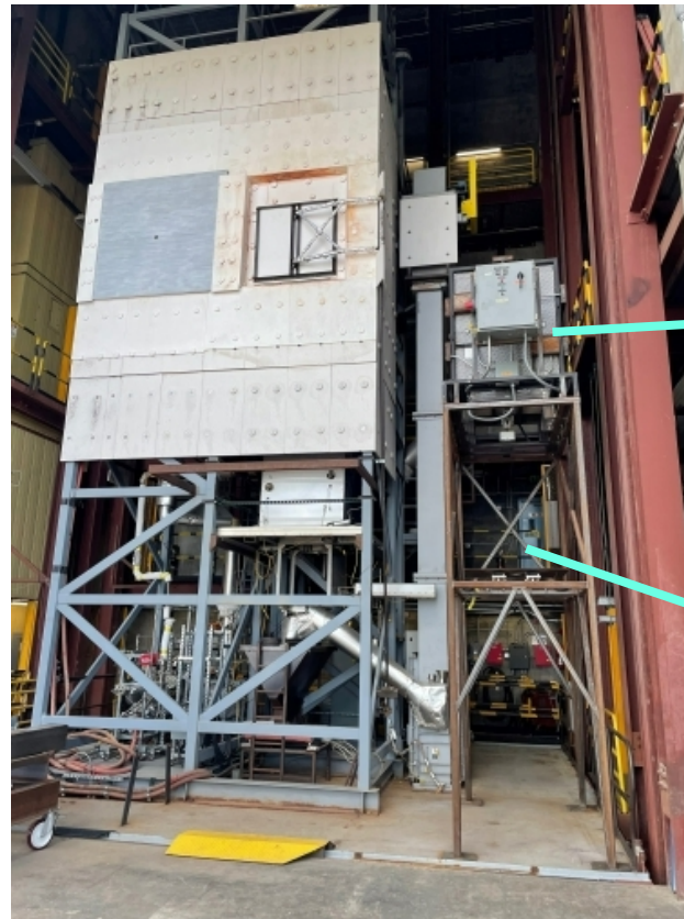
bucket lift and test stand next to falling particle receiver
