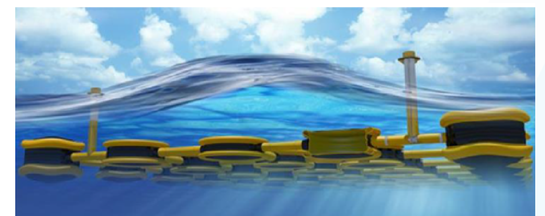
Communicating volume clusters, interconnected through PTOs with integrated resonance adjustment
