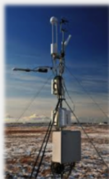
Eddy Correlation Flux Measurement System: Turbulent fluxes of momentum, sensible heat, latent heat, and carbon dioxide
