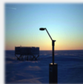
Total Precipitation Sensor: Precipitation, temperature and wind speed
