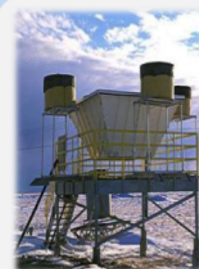
Radar Wind Profiler: Wind profiles and backscattered signal strength between 0.1 km and 5 km and virtual temperature profiles between 0.1 km and 2.5 km.
