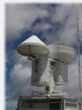
RADARS: Ka/W-band Scanning Cloud Radars: Fully polarimetric dual-frequency system with horizon-to-horizon scanning capability out to 50 km X (Barrow) or C (AMF3)-band Precipitation Radar: Volume scans out to 100 km
