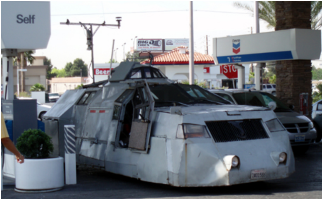
The TIV (Tornado Intercept Vehicle) built from a Ford F-450 (2006) Creative commons Wikimedia Creative Commons Attribution 2.0 Generic license.
