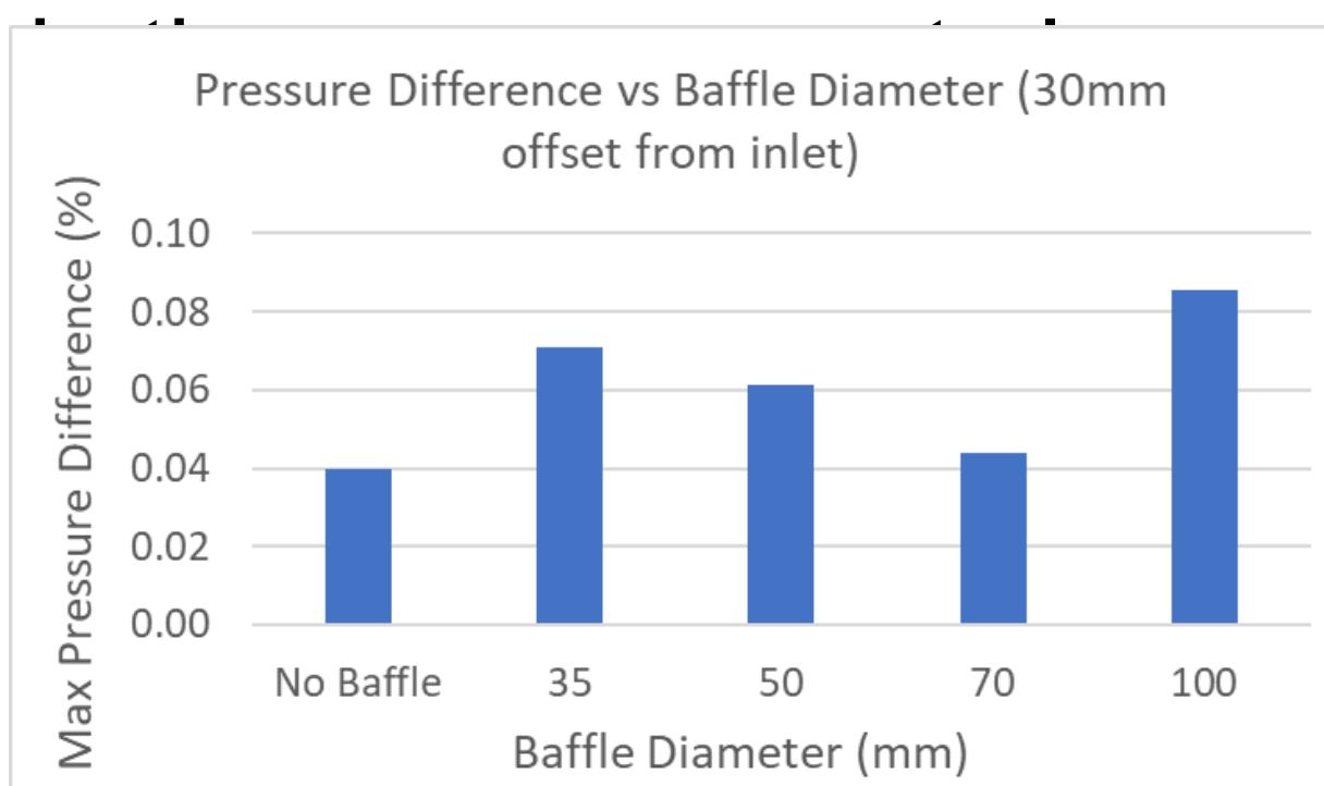
While holding the distance from the gas inlet constant, various baffle diameters were simulated.
