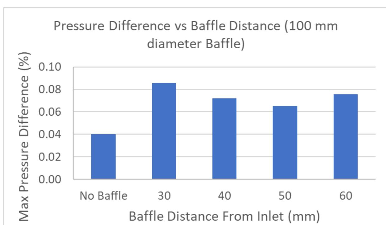
While holding the baffle diameter constant, various distances from the gas inlet were simulated.
