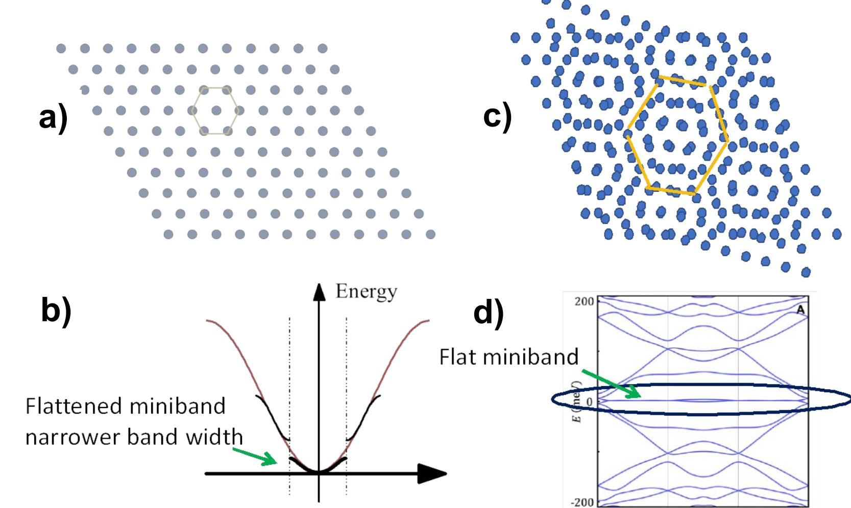
(a) Schematic representation of artificial graphene (AG). The blue dots form a honeycomb structure, as indicated by the yellow lines (b) Formation of flattened mini-band with a narrow band width. (c) Twisted bilayer AG with a twist angle of 15°. (d) Expected flat miniband formation in twisted bilayer AG.
