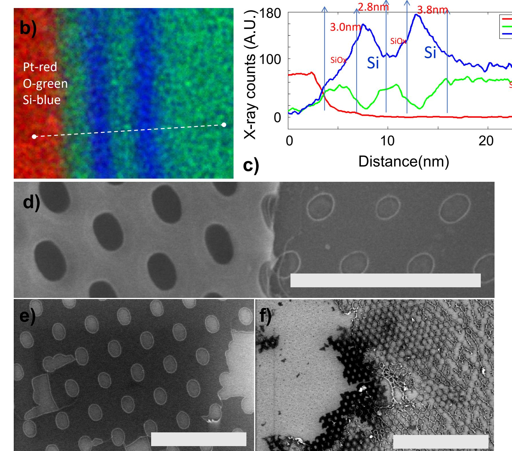
a) Cross-section TEM, b) EDS mapping and c) EDS line profile of transferred Si nanomembrane on Si nanomembrane. SEM image of d) 90° twisted-bilayer Si nanomembrane before cleaning (scale bar 1μm), e) transferred nanomembrane on SiO<sub>2</sub> after cleaning at 50,000 magnification (scale bar 1μm) and f) 10,000 magnification (scale bar 5μm).
