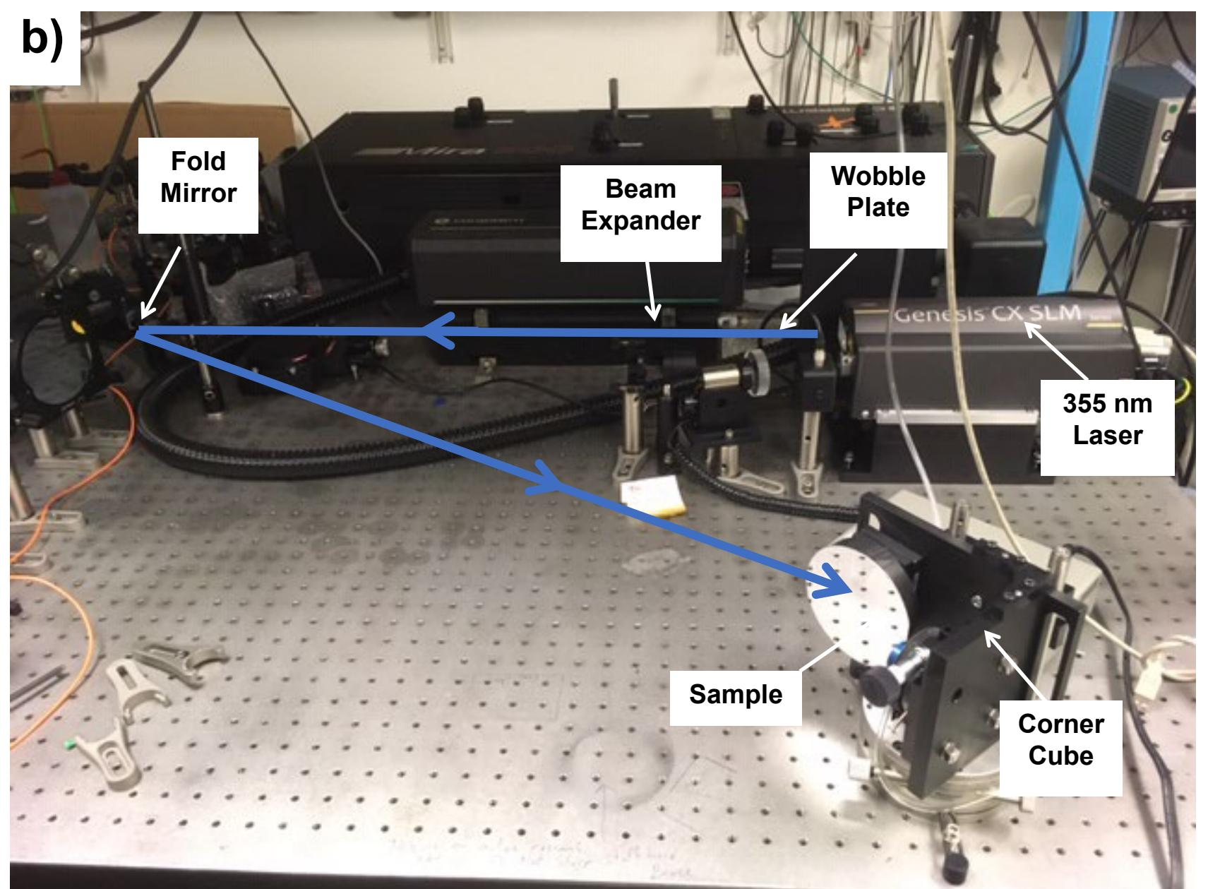
Schematic of a) the transfer printing process to fabricate twistronics superlattice and (b) the simple Lloyd's Mirror setup utilized in interferometric lithography.
