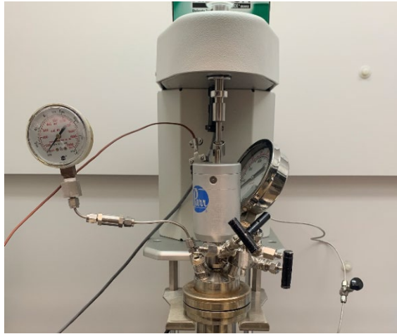
Bench-scale hydroprocessing to screen catalysts and process conditions
