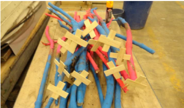
Figure 4 : Roughly half of the larger debris pieces were fitted with artificial root wads.
