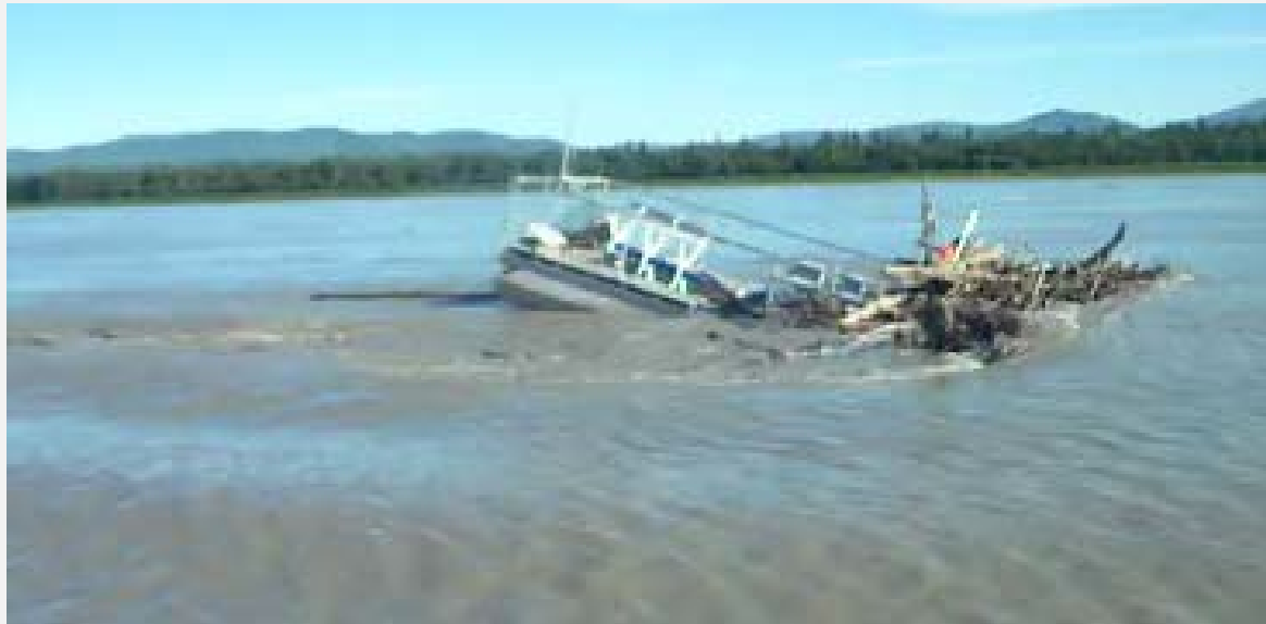
Debris accumulation on 25 KW New Energy turbine at Eagle AK [2]
