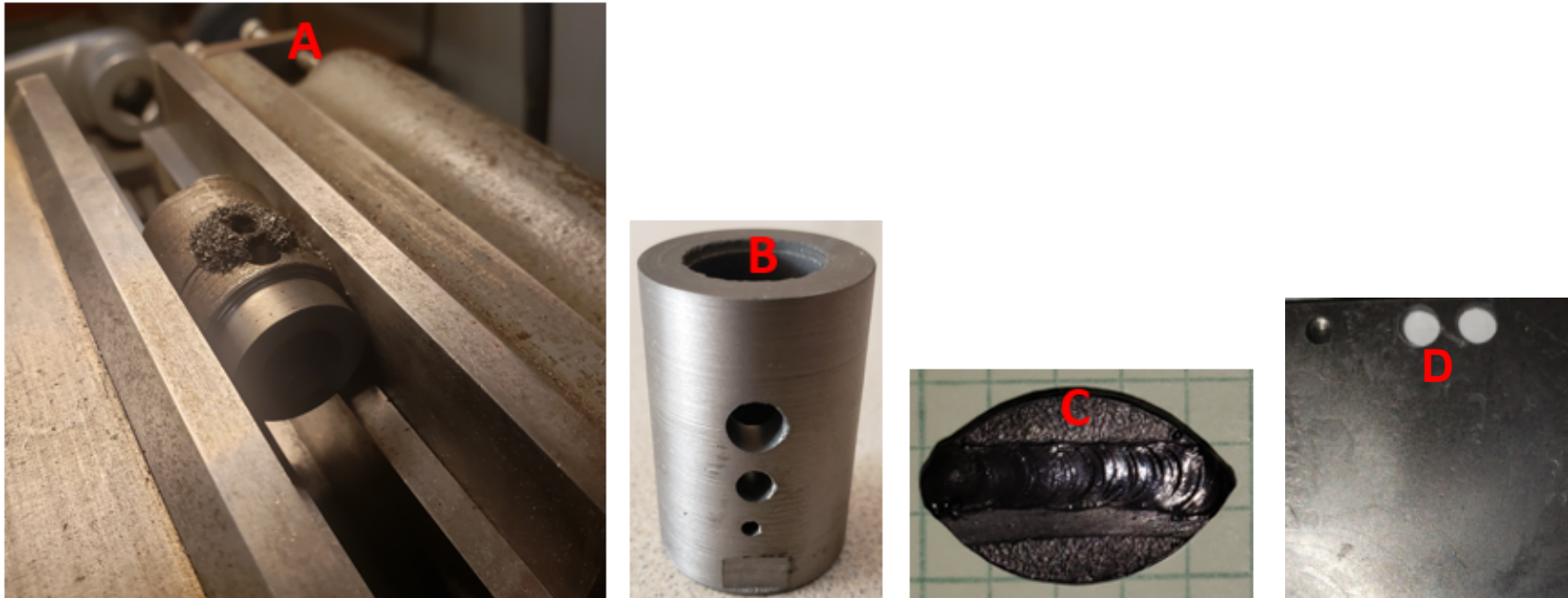
A. Rotational lathing of a RHEA tube. B. Drilled and lathed RHEA. C. RHEA-to-RHEA welding. D. RHEA drilling.
