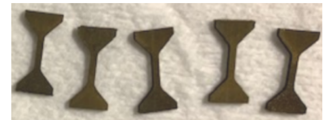
NbTaVW RHEA Type A dogbone specimens printed via the LENS machine.
