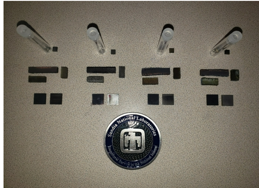
Multiple RHEA composition pieces printed using the Laser Engineered Net Shaping (LENS) approach [Smith, 2016].
