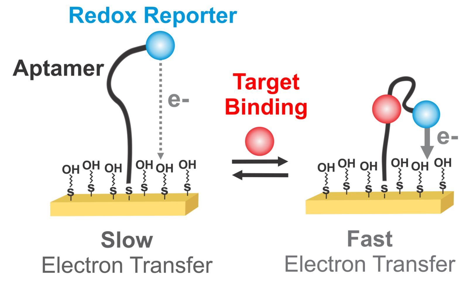
Typically, electrochemical aptamer based sensors consist of a **redox reporter-modified aptamer sequence** attached to a gold electrode via a surface assembled monolayer
