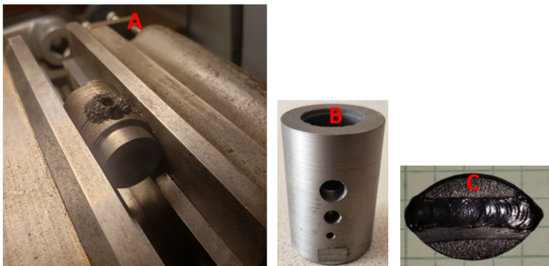
Figure 2: A. Rotating lathe of RHEA tube. B. Drilled and lathed RHEA. C. RHEA to RHEA welding.
