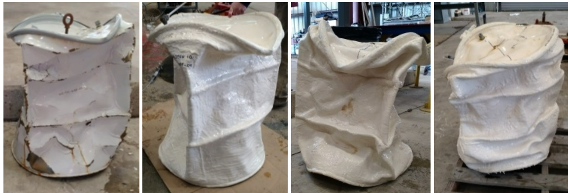
Hydrostatic compression test results - Full-size waste drum
