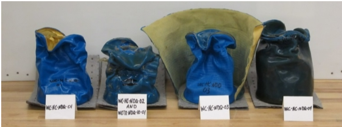
Hydrostatic compression test results -- 1/4-scale waste container
