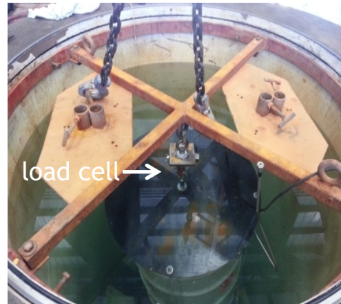
Hydrostatic compression test for full-size waste drums
