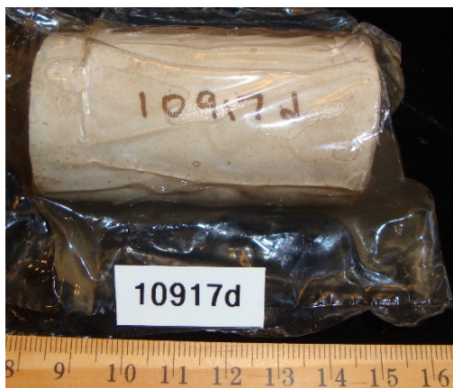
Figure 5. Grossite CAPC cement sample post-hydrothermal treatment.
