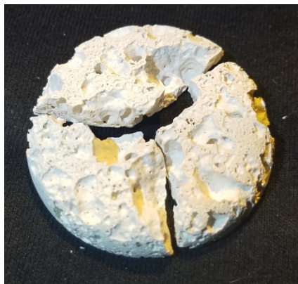
Figure 1. Standard APC cement sample with large voids.
