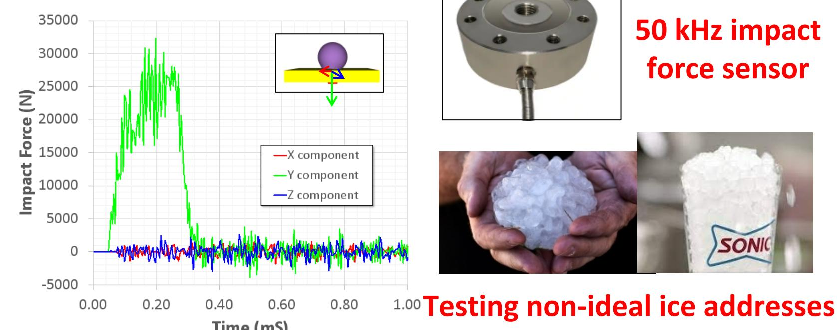
Simulated impact force vs. time produced by hail ice will be validated against measurements
