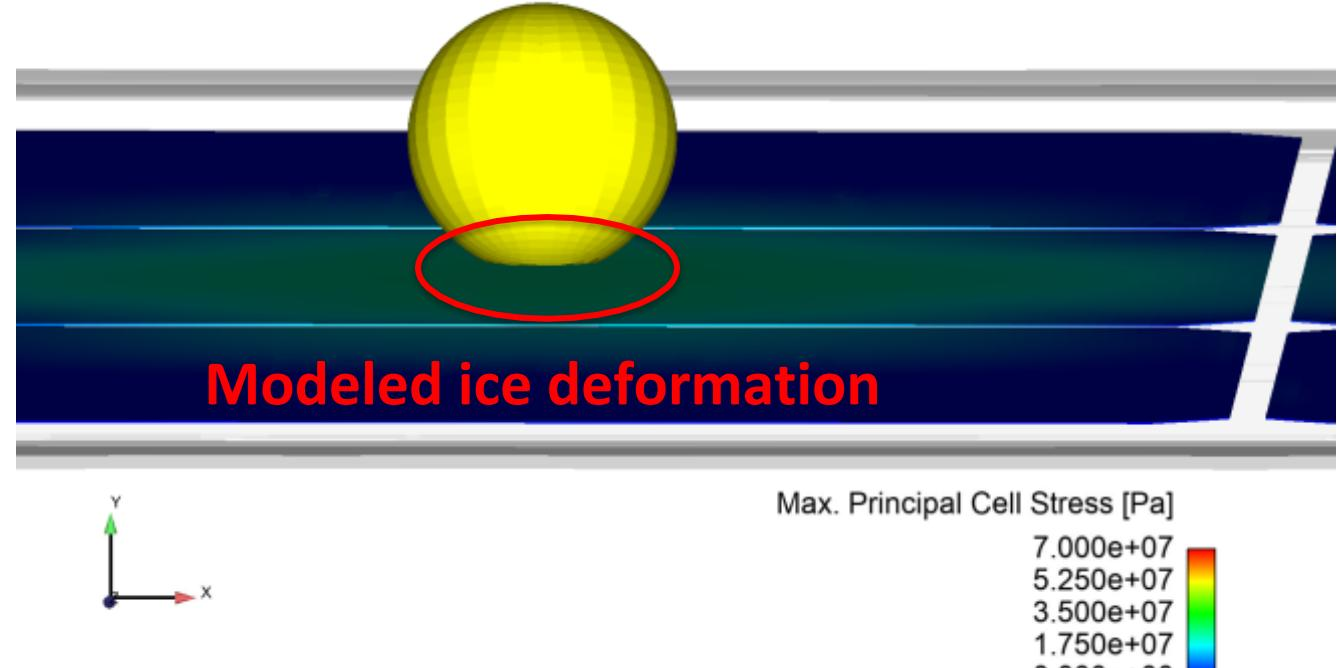
A hail impact vs. PV module simulation was successfully demonstrated using the SIERRA solid mechanics code
