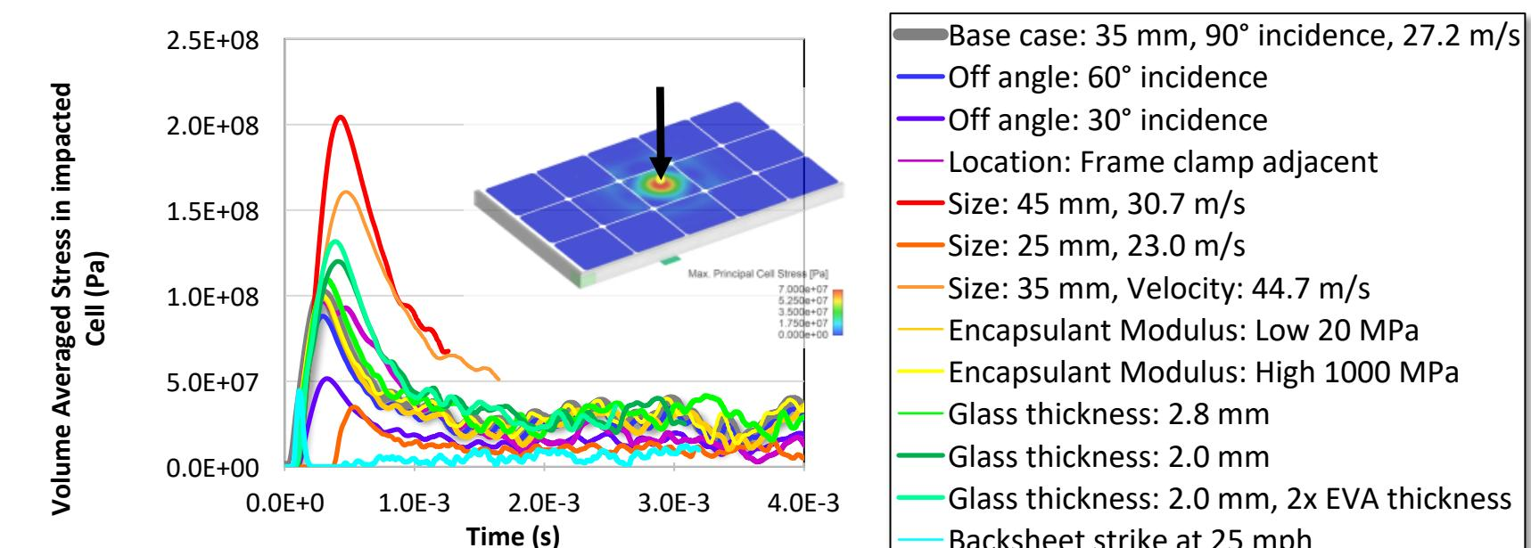
Initial parametric studies show how cell stress during impact is affected by hail and module characteristics
