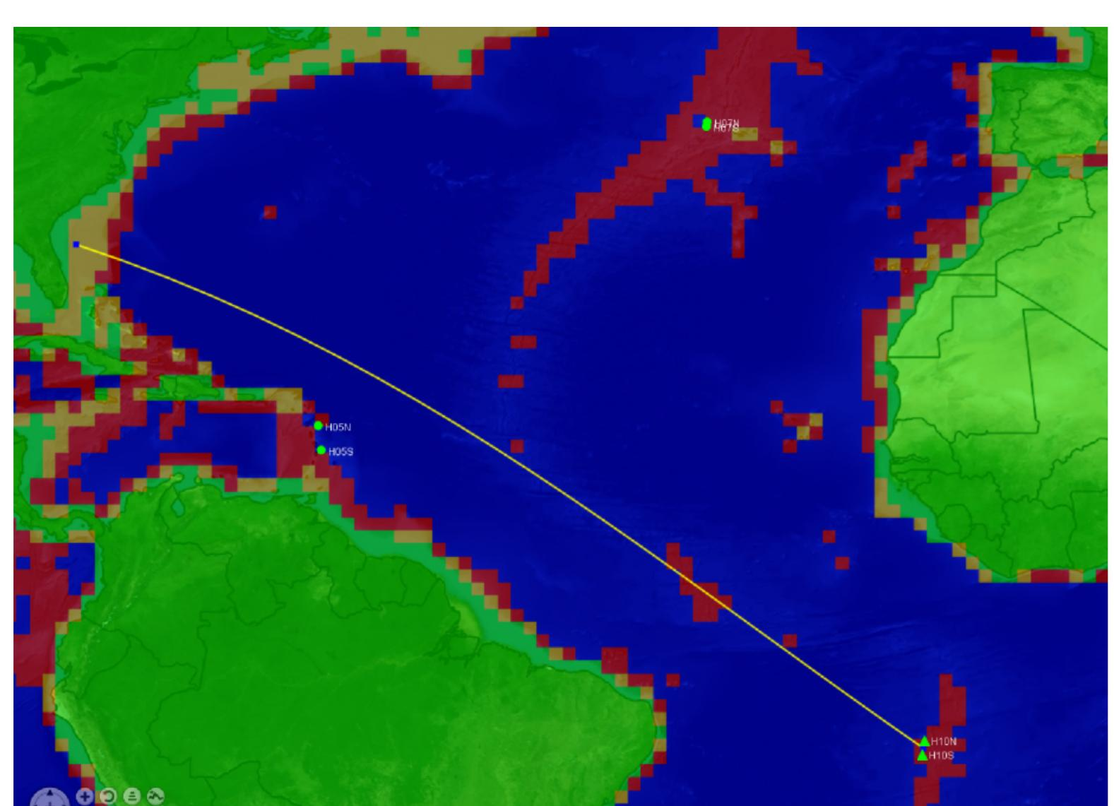
The path-weighted estimate of attenuation agrees well with several RAM simulations over the radial path ranging out to over 8000 km of distance.
