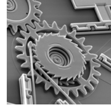
Above: gears in contact within MEMS device. From sandia.gov/media
