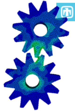
Above: gears in contact within MEMS device. From sandia.gov/media
