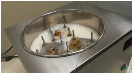
Fig.2. Adopted setup to measure thermal conductivity at different temperatures.
