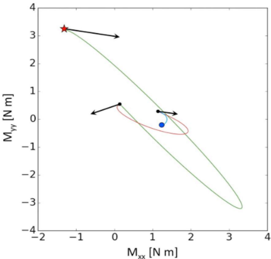
Example model space trajectory of two model parameters, based on kinetic and potential energy
