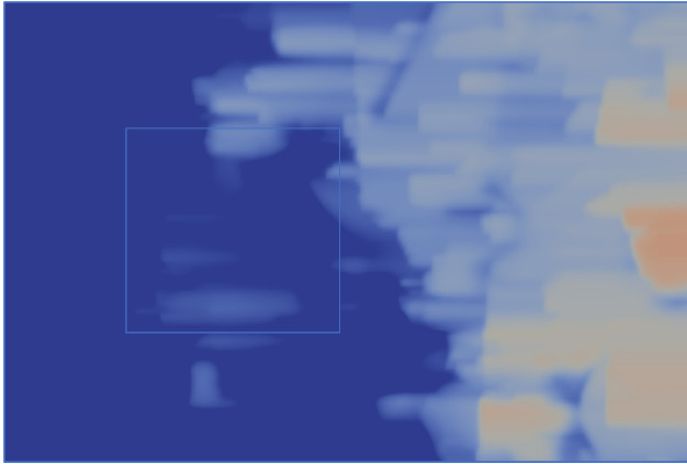
Fig. 3. Overhead view of dispersion of ^{129}\text{I} concentrations in a simulation of a homogeneous shallow aquifer above a hypothetical repository in crystalline rock. The rectangle shows the extent and location of the repository 560 meters below the aquifer. Warmer colors show higher ^{129}\text{I} concentrations.
