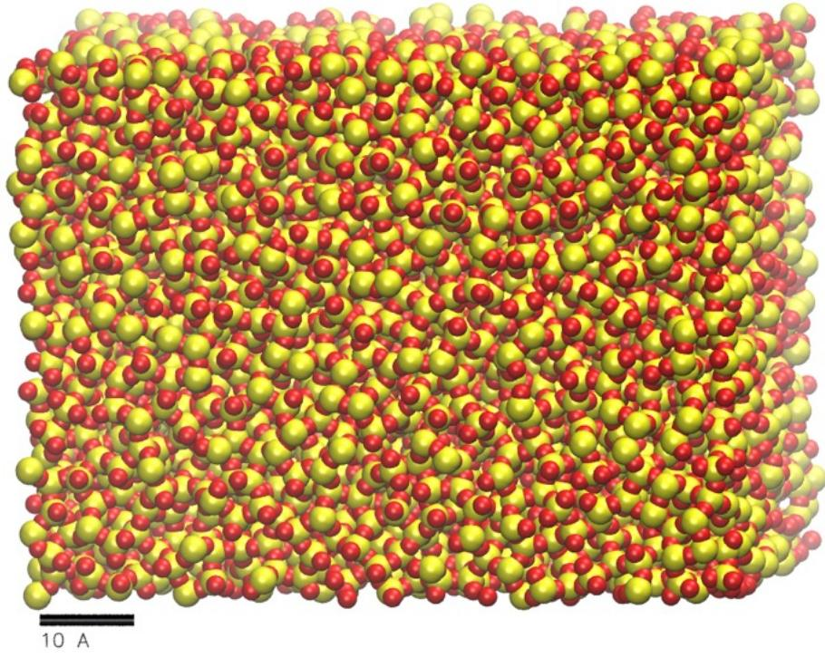
MD simulation from LAMMPS of silica (SiO<sub>2</sub>) Image from J.M.D. Lane.
