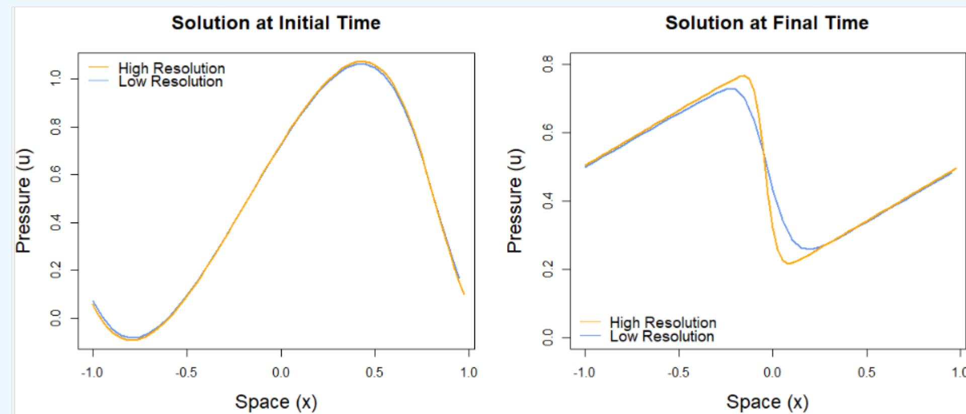
By treating high and low fidelity solutions as functionals we can apply functional regression to predict high fidelity solutions from low fidelity inputs at reduced computational burden.
