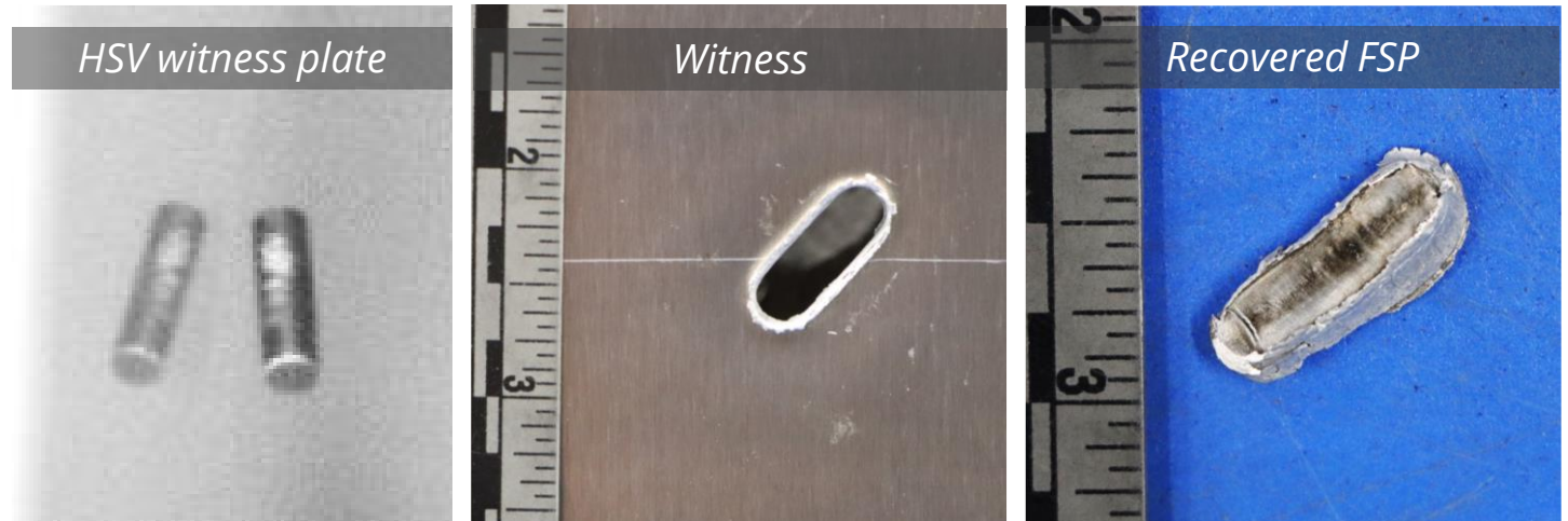
Aluminum on aluminum (1/8" plate) at 1.23 km/s side-on FSP
