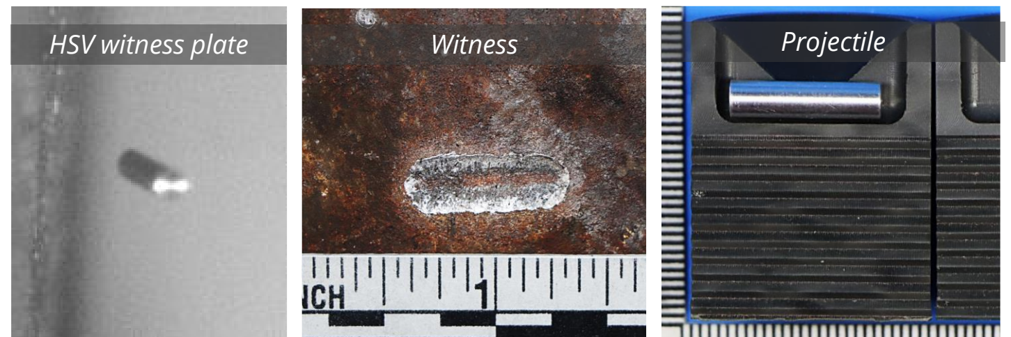
Aluminum on Steel (1/4" plate) at 1.24 km/s side-on FSP
