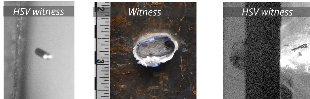
Tungsten on steel block at 1.22 km/s side-on FSP
