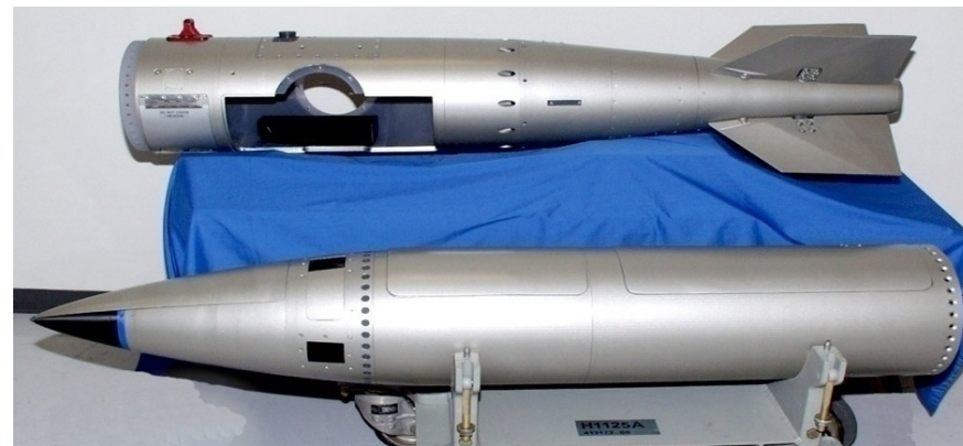
Full scale additive weapon mock-up
