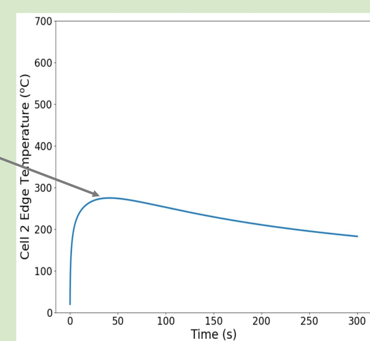
Thermal evolution of  $T_c(t)$  (Heat release turned off)
