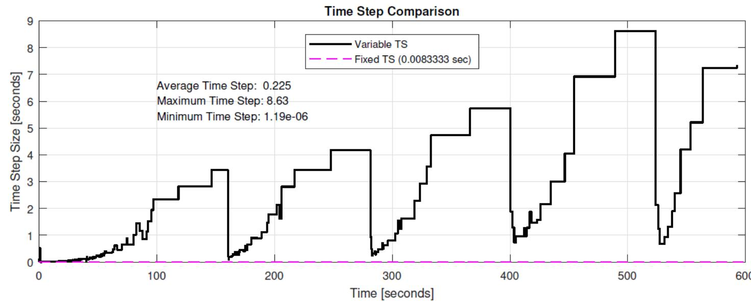
Comparison of time step size for variable time step and fixed time step methods.
