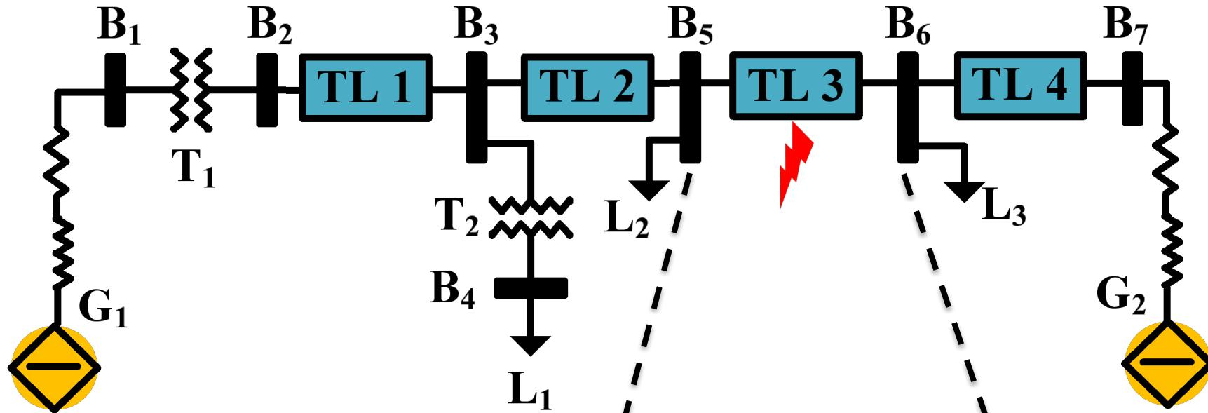
Measurements for the TW relay were taken at Bus B5, using single-ended protection scheme
