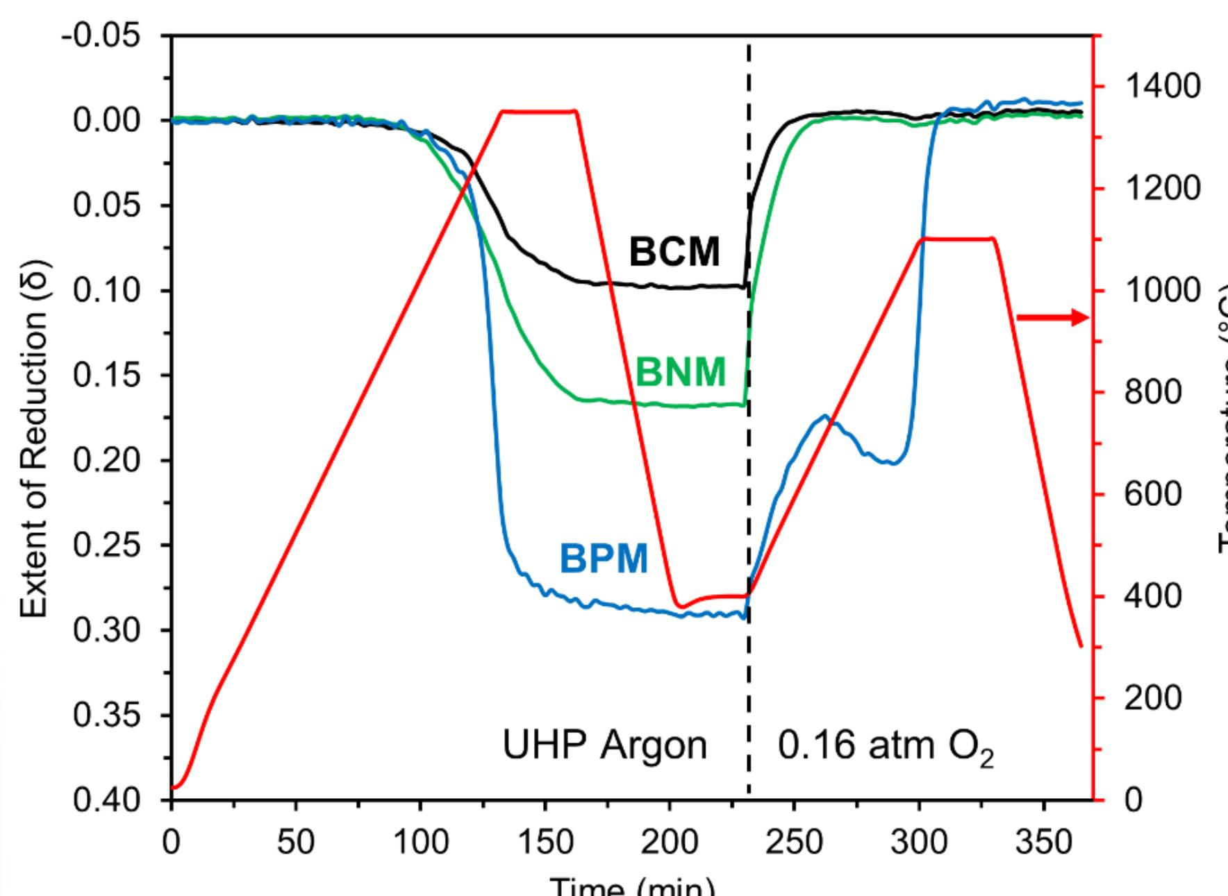
BCM, BNM and BPM showed reduction under Ar at 1350 °C ( $\delta = 0.08\text{-}0.28$ ) and oxidation at 1100 °C under air ( $\delta=0$ ), with BCM showing the smallest reduction. BPM shows the largest reduction, suggesting possible  $\text{Pr}^{3+}/\text{Pr}^{4+}$  reduction, oxidation of BPM appears to also show the two-step oxidation of  $\text{Mn}^{+3}$  to  $\text{Mn}^{+4}$  and  $\text{Pr}^{+3}$  to  $\text{Pr}^{+4}$ .
