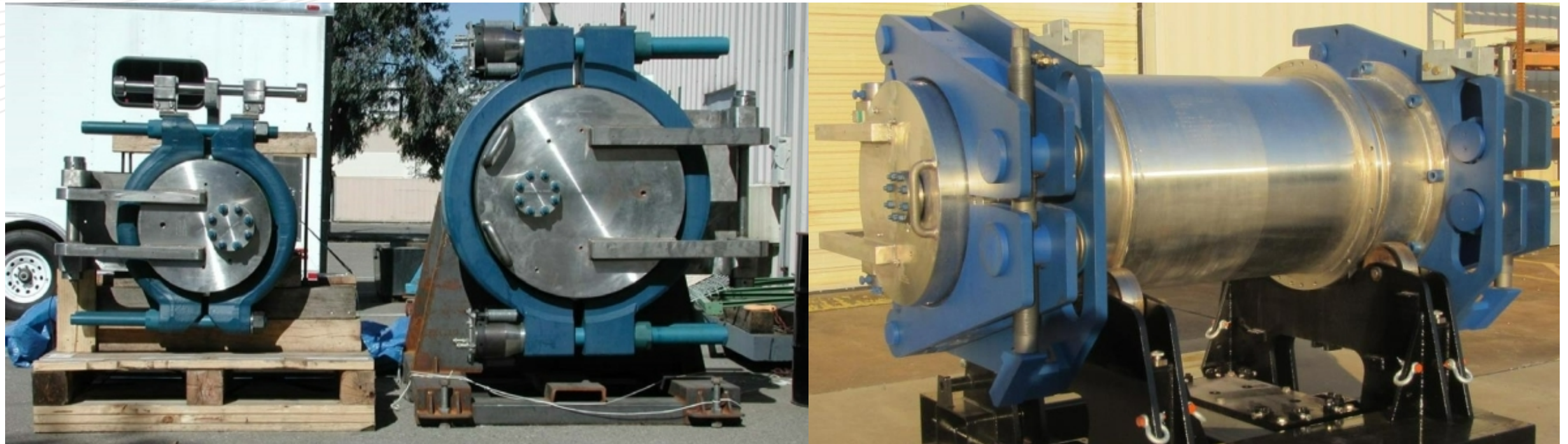
The P1 and P2 vessels with the two piece door clamping system
