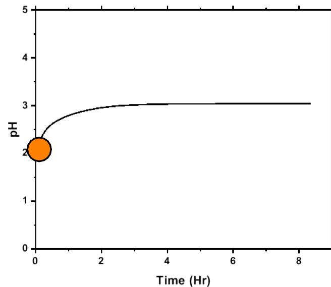
Decrease in pH, increases local cathodic reactions, causing for a subsequent pH rise
