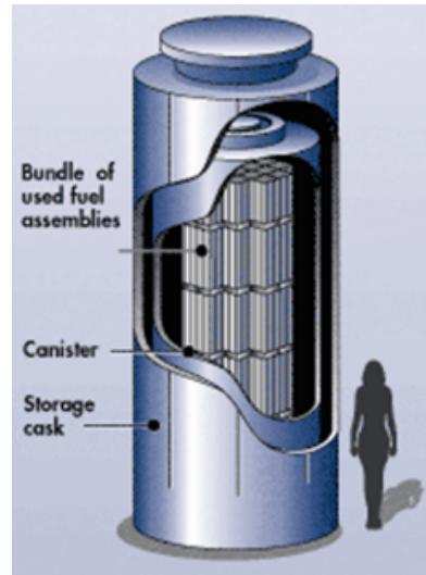
SNF Canister inside concrete overpack
