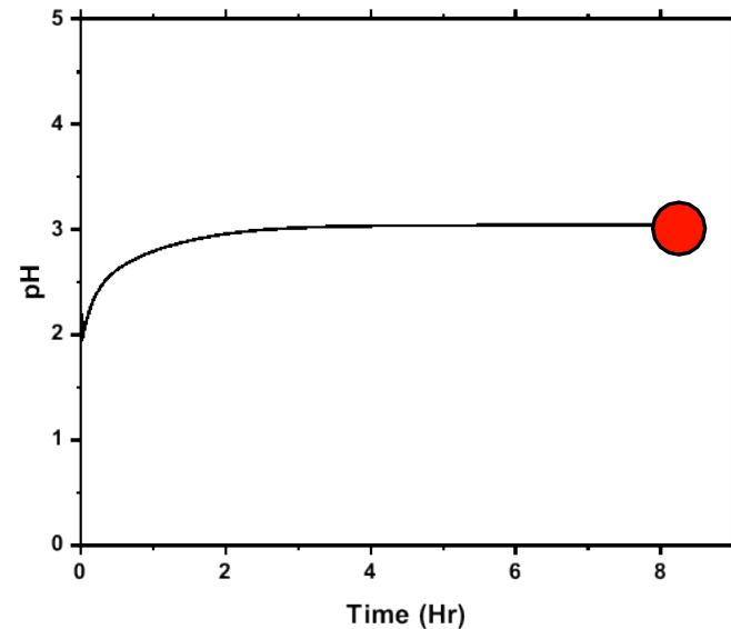
**'High' pH due to significant contribution from local cathodic current**
