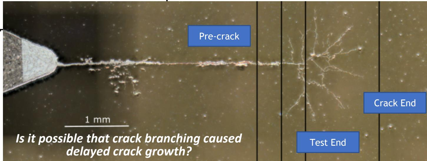
*Is it possible that crack branching caused delayed crack growth?*
