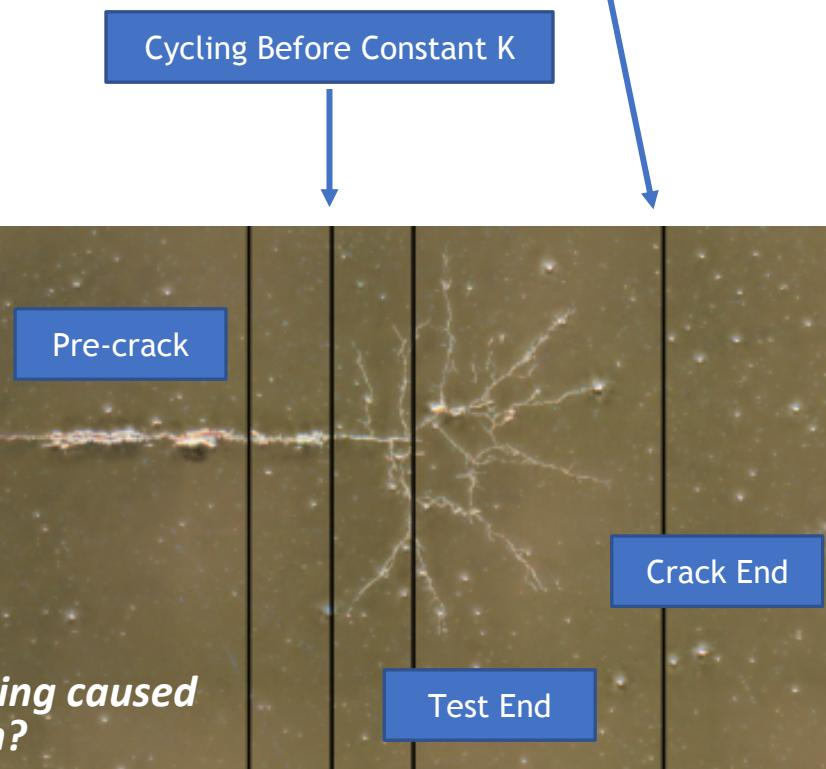
*Is it possible that crack branching caused delayed crack growth?*
