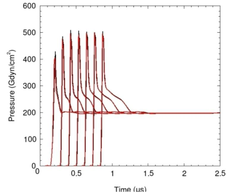
Sensitivity to equilibrium assumption depends on velocity - overdriven detonations are less sensitive
