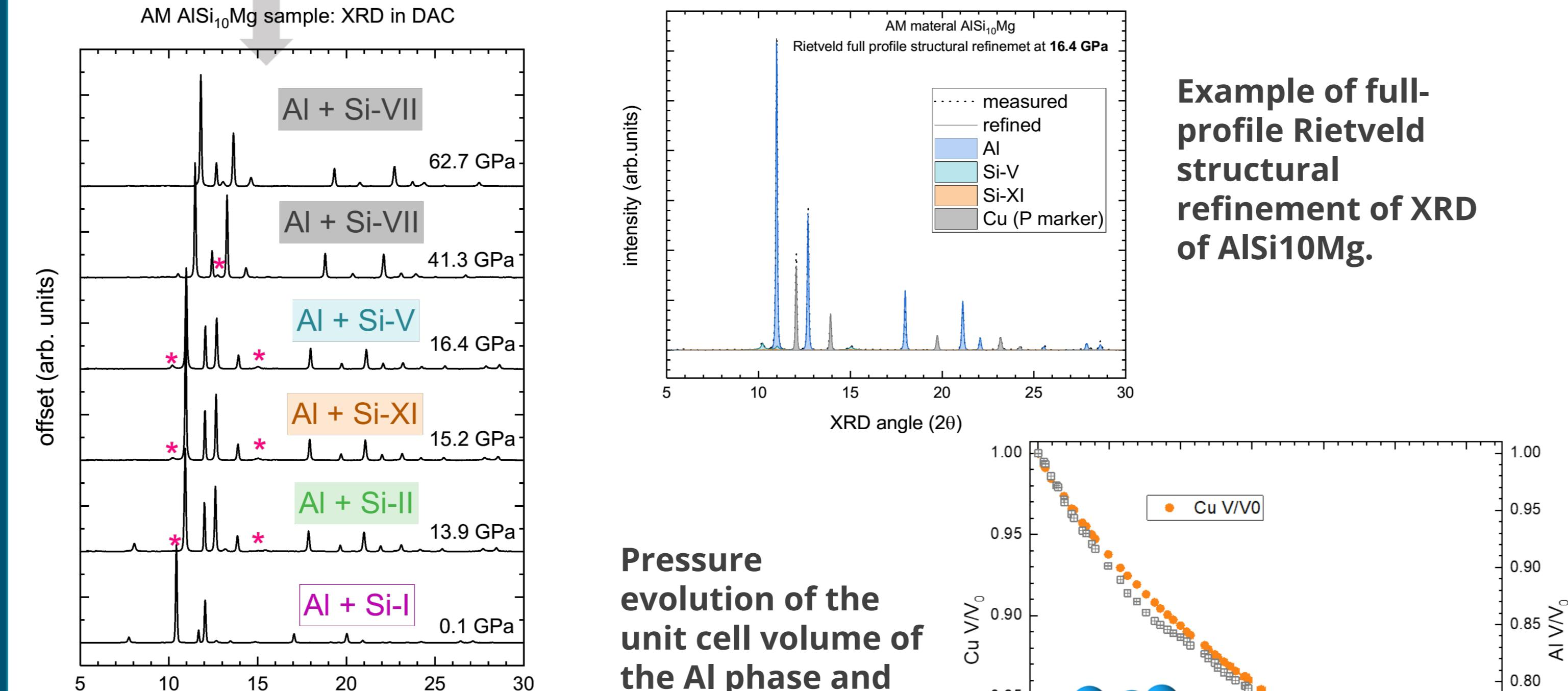
Example of full-profile Rietveld structural refinement of XRD of AlSi10Mg.
