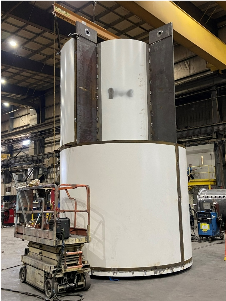
Vertical Cask Mockup: Steel-Concrete-Steel Vertical Cask Carcass at the Manufacturing Facility
