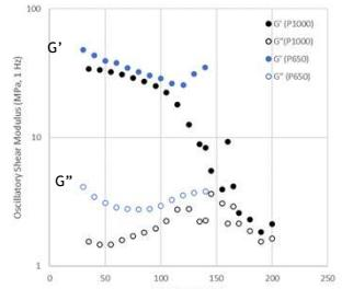
As the soft domain molecular weight is decreased from P1000 to P650 to P250, the modulus and glass transition temperature ( $T_g$ ) increase. Viscoelasticity and energy damping are maximized near  $T_g$  where the storage and loss shear moduli are both significant.
