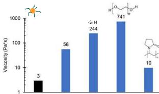
Of all polymers, surface modification with PVP creates best compatibility with polyurea precursors, as measured through viscosity of the particle-filled suspension
