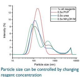
Particle size can be controlled by changing reagent concentration
