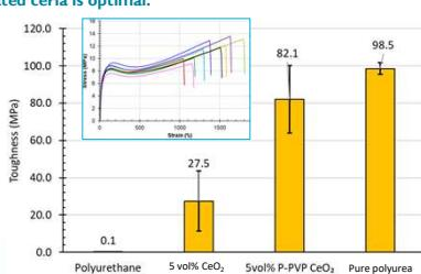
Poor particle-polymer compatibility results in degraded composite toughness and maximum tensile strain when tested in tension
