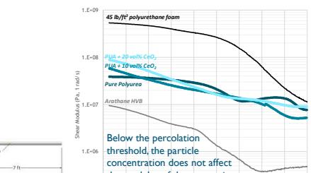
Below the percolation threshold, the particle concentration does not affect the modulus of the composite significantly.
