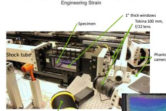
Shock tube imposes a mach 2.5 blast of air on a 4x4 inch, 1 mm thick plate of aluminum, covered with a 1.5 mm thick polyurea sample and deflection is measured using DIC.
