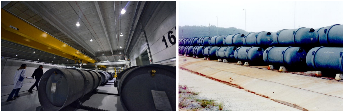
Figure 2. 48-inch containers are used to store and transport natural and depleted \text{UF}_6 . Our Limbo dataset includes three models: the 48Y (left) and 48X are used to store and transport \text{UF}_6 , while 48G containers (right) are used exclusively for storage. Credits: IAEA, 2015 (left); United States Department of Energy, 2016 (right).
