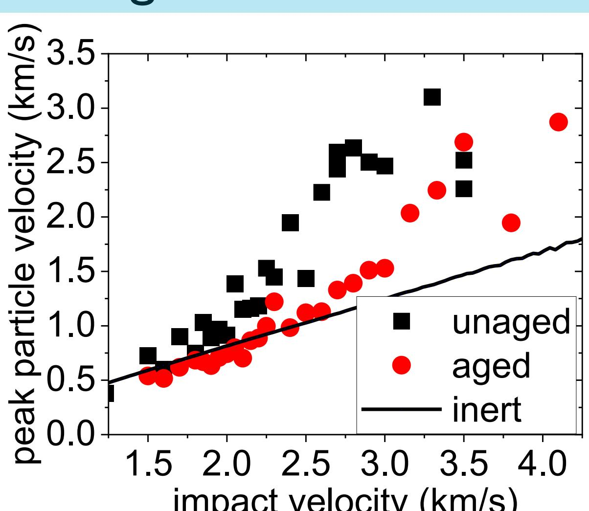
Pentaerythritol Tetranitrate (PETN) is seen to coarsen and coalesce with increased porosity with thermal aging. This microstructural effect is shown to decrease sensitivity, increasing the impact velocity required to force a deviation from a simulated inert response. The large variance in peak particle velocity near 2.5 km/s is indicative of detonation. Such sampling using > 100 explosive targets is made possible due to the high-throughput nature of the experimental platform.
