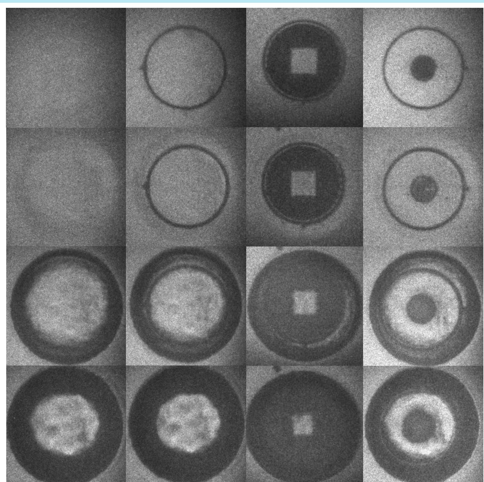
Imaging of parylene C flyer launch with various cut-outs for flyer shaping. Frame exposure is 10 ns with 25 ns interframe time. PDV shows no difference between non-cutout and cutout flyers, indicating tensile strength plays little role in these plastic flyers.
