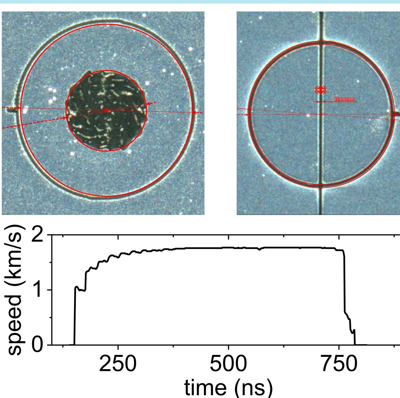
Femtosecond laser cutting of flyer optic allows for custom shapes including arbitrary shock geometries and fragmentation arrays. PDV trace is representative for annular section of “donut” flyer. No signal is present when centered on donut hole. Imaging of both bisected and donut flyers show parylene C launch of pre-cut shapes.
