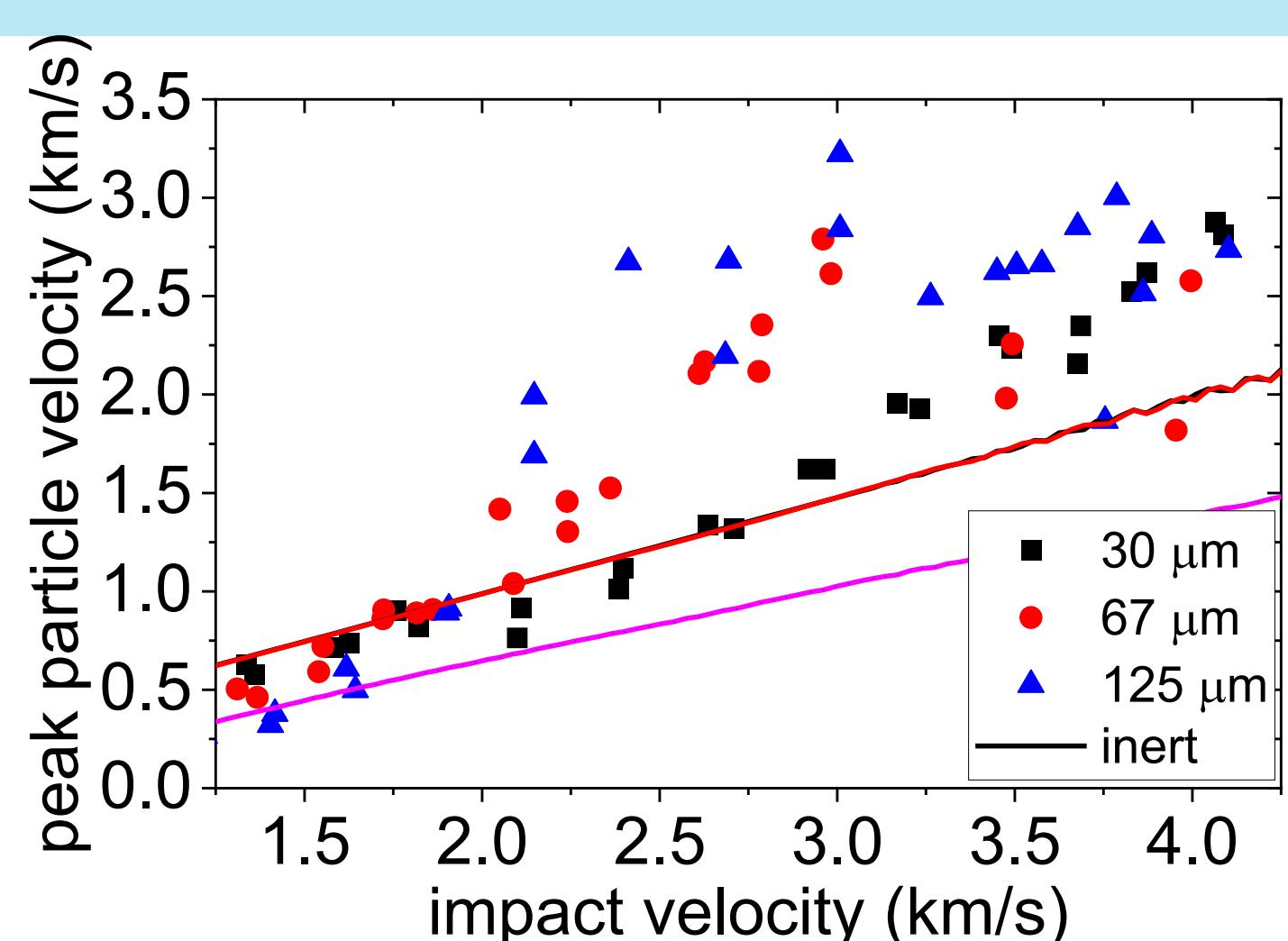
Utilizing multiple samples of varying thickness, allows for measurement of buildup to detonation similar to cutback experiments. PETN is seen to be just beginning to react at a depth of 30  $\mu$ m, with deviation from inert simulation gradually beginning at 3 km/s. Initiation threshold is determined to be around 2.4 km/s by the 125  $\mu$ m thickness.
