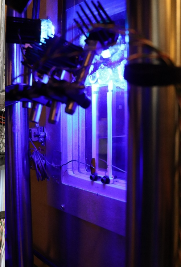
IR transparent window and lighting for DIC
