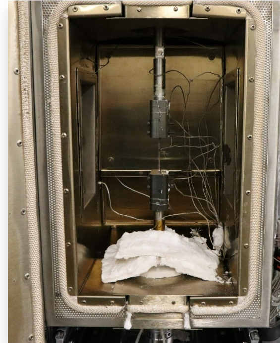
Convective furnace on MTS servo-hydraulic load frame
