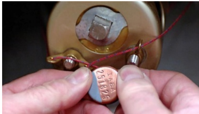
Figure 1: CAPS metal seal, image: IAEA, 2020.
